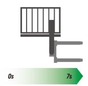
**Traverse Speed** Complete full traverse in 7 seconds.
